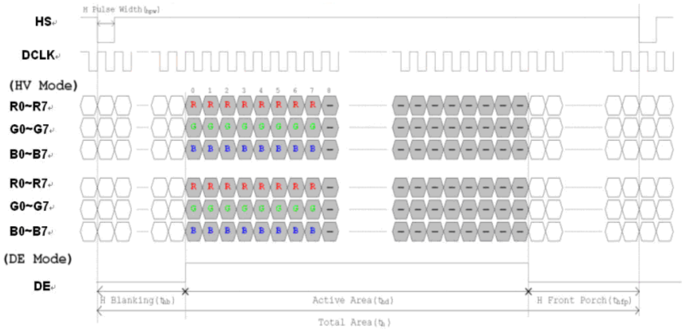
Figure 5: Horizontal Input Timing Diagram
